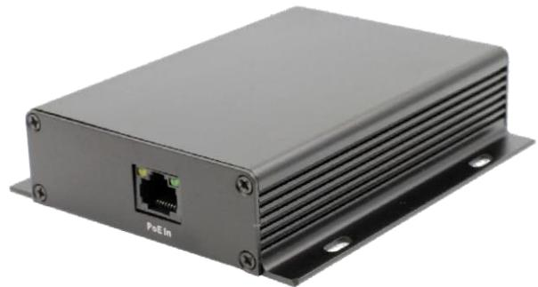
**PoE Ethernet Extender** is a high-speed Ethernet transmission device. It transmits Ethernet and PoE signal up to 500m over 2-wire cable such as Cat5, coaxial cable, telephone line and power line. The max physical bandwidth can reach 200Mbps. This device supports both PoC and PoE function.
